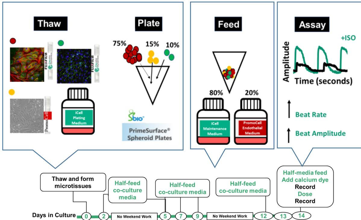
**Figure 1: A Schematic Showing Different Steps Involved in Assembling the Triculture Microtissue and Timeline of the Workflow From Day 0 Until Ready for Assay.**
